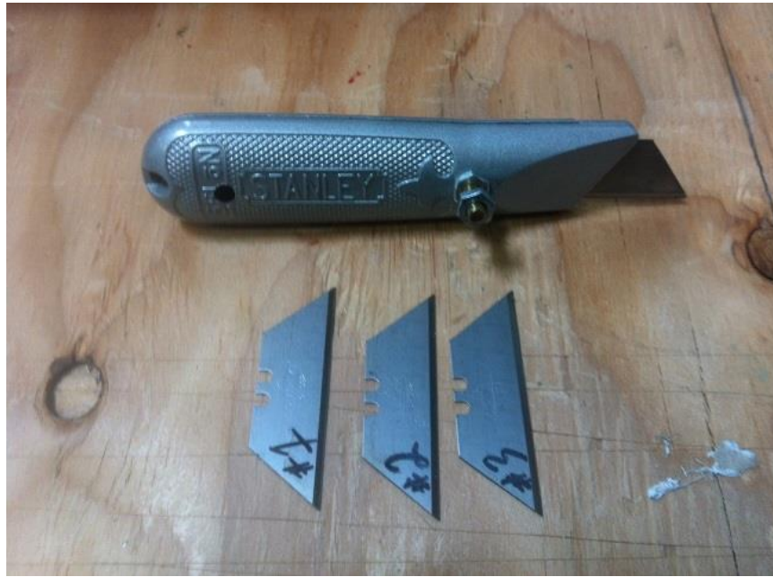
Photo No. 1 Test rig knife with new blades for each specimen
